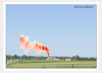
The image shows a coal mine ventilation shaft which emits methane. Methane is invisible to the human eye, yet the HySpex camera reveals the plume emanating from the left shaft. Darker colours correspond to a higher atmospheric methane content.
